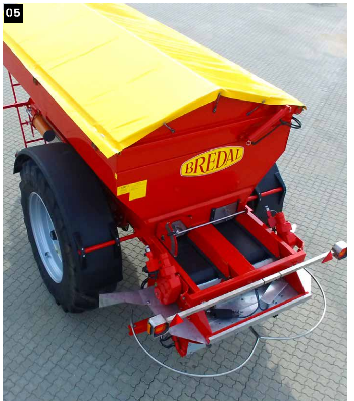
1 > BREDAL F8 2 > SPREADING SYSTEM with 2 belts, 2 back doors and 2 independently operated downchutes 3 > ELECTRICALLY OPERATED DOWNCHUTE 4 > SENSOR 5 > F8 FROM ABOVE 6 > SCALE FOR REAR DOOR
