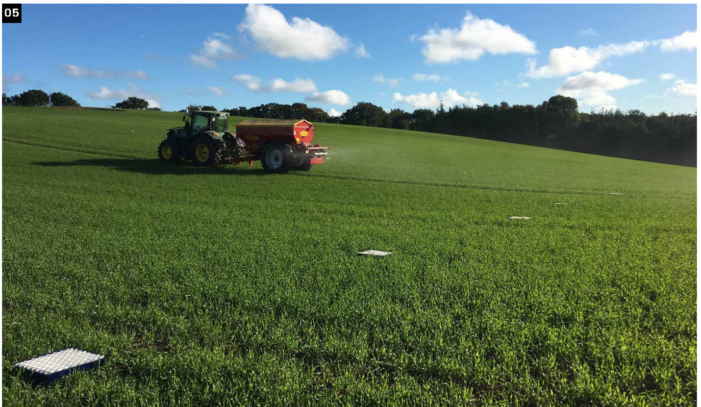
1 > A SIEVE TO MONITOR GRAIN SIZES 2 > CALIBRATION KIT 3 > MEASURING TUBE 4 > BREDAL TEST KIT The test kit includes plastic trays with dividers, measuring tube, funnel, granule strength tester and a sieve 5 > SPREADING TEST IN THE FIELD with Bredal machine and Test kit (trays positioned on the field)
