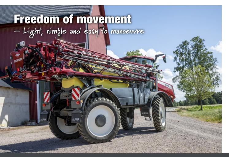
The ALPHA evo has been designed with an effective weight distribution between front and rear axles, with slightly more weight on the front (59% on front with a TWIN FORCE 30 m boom) to strike a perfect balance between driveability and minimal compaction.
