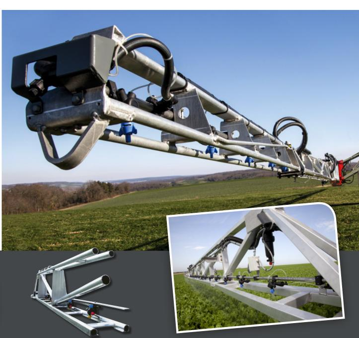
Aluminium boom structure (TR4 24 to 33 m)
