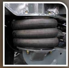
**Driving comfort: Three point suspension**The HELLIOS III features a pneumatic three point suspension on its chassis:
