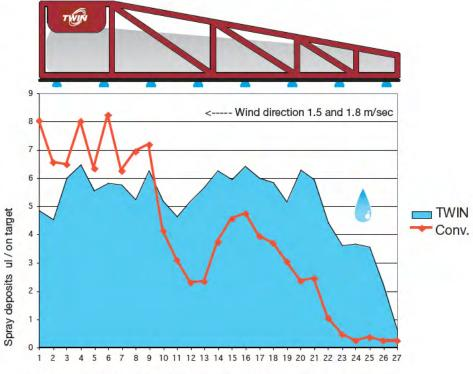
Sample location (at 0.25 m intervals) from sprayer's wheel to swath edge
