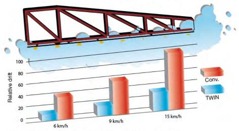
Nozzle: ISO-F025 @ 2 bar. 6 km/h - 160 l/ha. 9 km/h - 110 l/ha. 15 km/h - 65 l/ha. Wind velocity: 2-4 m/sec. (HARDI INTERNATIONAL A/S, 2003)
