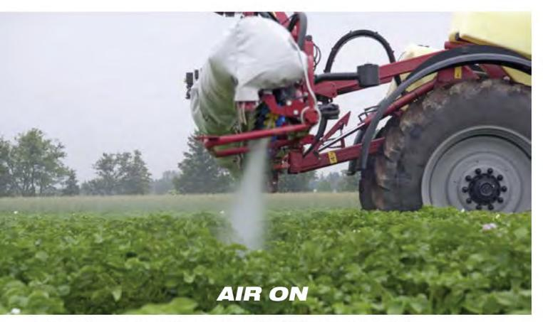
In this situation the wind is about 8-9 m/s, and the drift is strongly reduced with TWIN air on.
