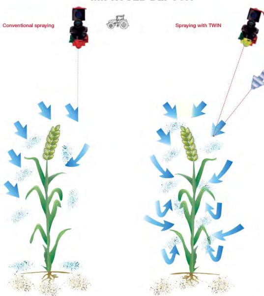
When fine / medium spray qualities are sprayed with conventional sprayers without air assistant, the deposit on the backside and in the upper area of the plant is higher. The finer droplets are hanging in the air.
